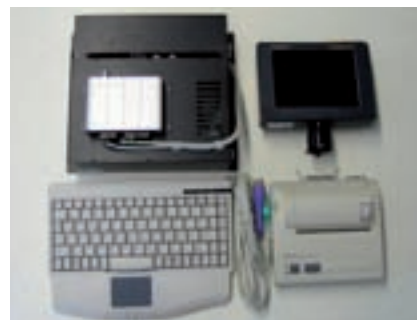
BC2 – Bordcomputer, Monitor, Tastatur, Drucker
