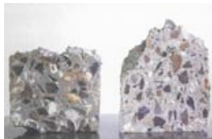
Fig. 24: Axial cross-section through the stream of concrete, left = blockage, right = flowing*
