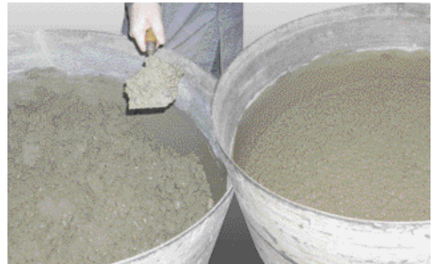
Fig. 7: Concrete before and after addition of plasticising admixture
