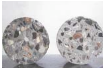
Fig. 25: Radial cross-section through the stream of concrete, left = blockage, right = flowing*
