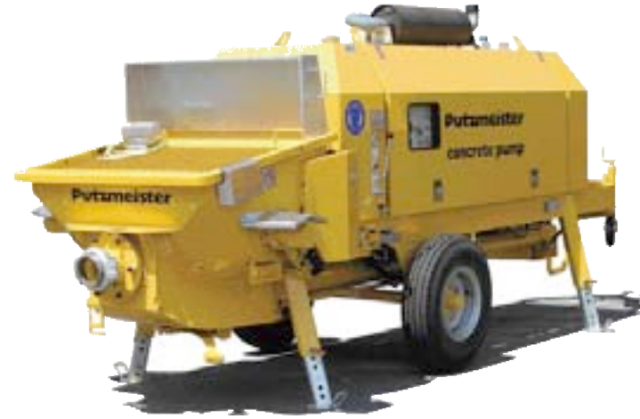
Fig. 29: Putzmeister stationary concrete pump BSA 1407 D
