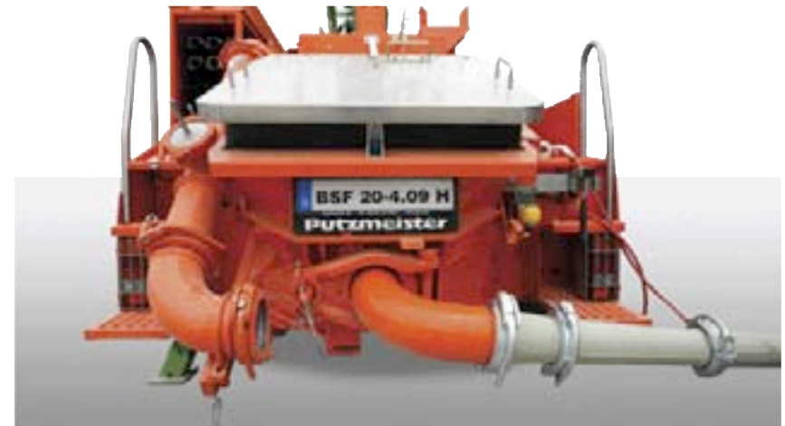
Fig. 30: Reduction from DN 150 to DN 65
