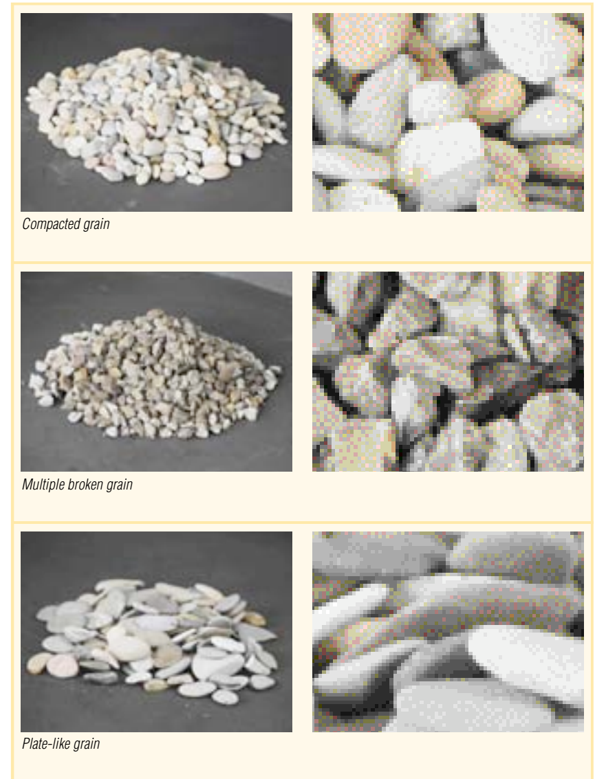
Fig. 5: Influence of the shape of the grain on the surface with the same volume
